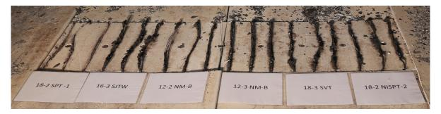
Figure 5.1: Photograph of the 18 cord exposures in the test room following Experiment 2. The placards identify the cord type.
